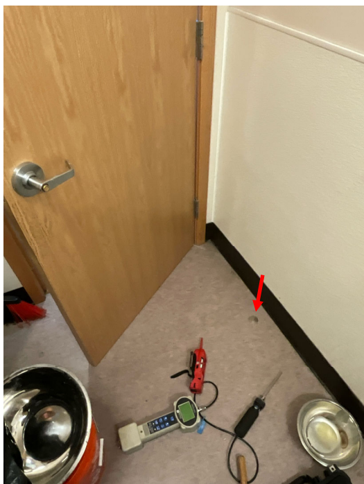
Photograph No. 01: View of newly installed vapor pin VP-1, located inside of the ELF Daycare building.
