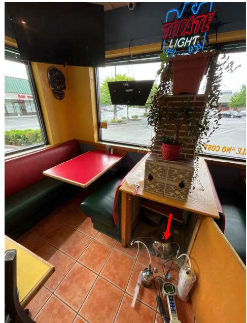
Photograph No. 06: View of newly installed vapor pin VP-6, under helium shroud, located inside of El Paraiso Mexican Grill building.
