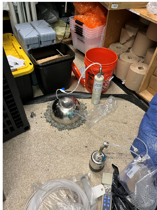
Photograph No. 02: View of existing vapor pin VP-2, under helium shroud, located inside of the Bliss Small Batch Creamery building.
