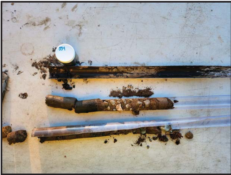
Profile of Soil Boring SB34 No Visual or Olfactory Evidence of Oil on Northern Property Boundary
