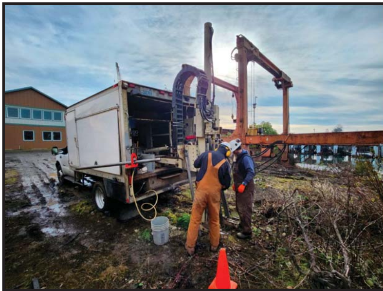
B&W Standard Probe Advancing the Direct-Push Probe at Location SB39
