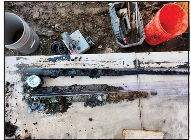
Profile of Soil Boring B38 Clear Presence of Oil (Identified as Hydraulic Oil)
