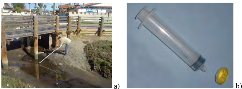
Figure 5: a) Dipper and extension pole used from a streambank. b) Syringe and filter used for dissolved nutrient samples
