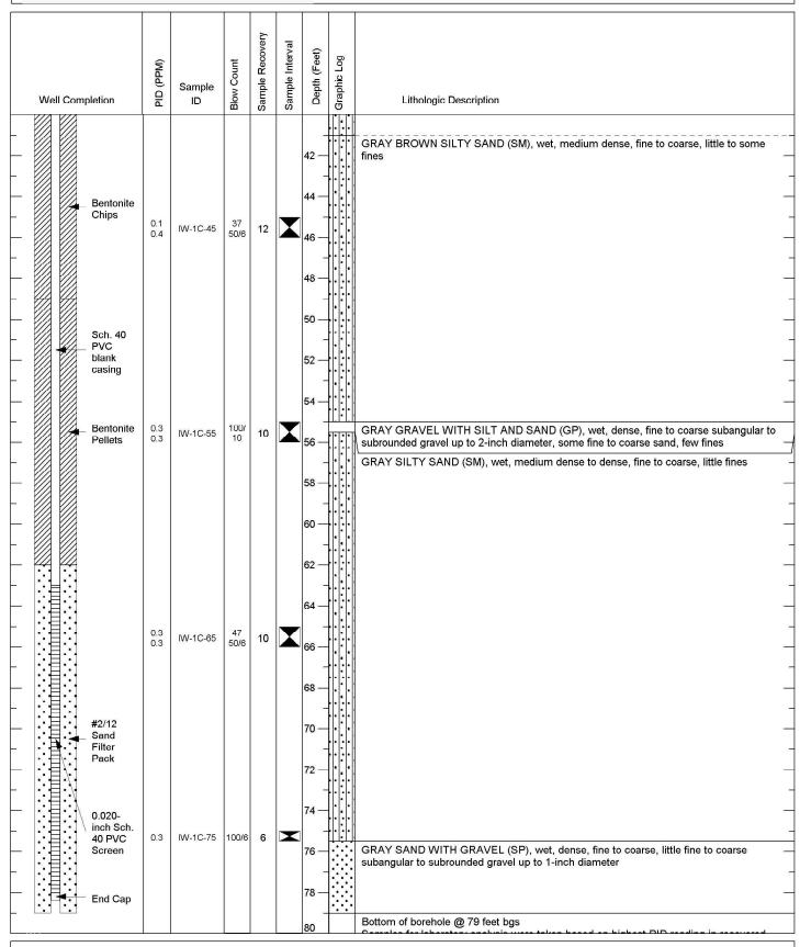
Logged By: RTM Notes: 140 lbs. Hammer w/ D&M Total Drilled Depth: 79
