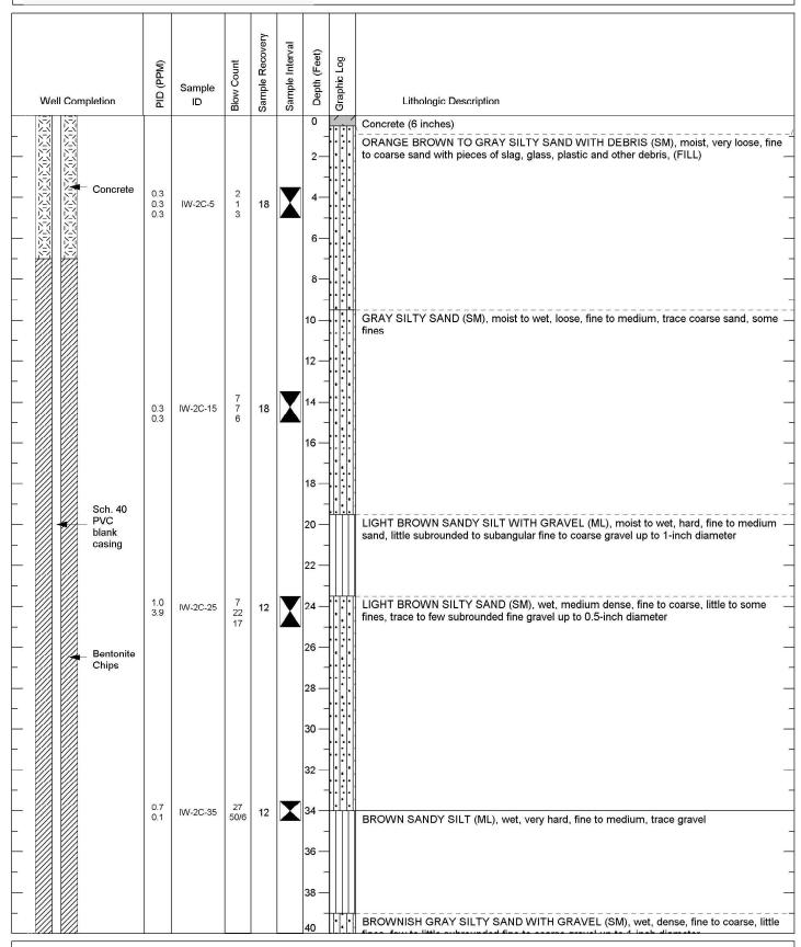
Logged By: RTM Notes: 300 lbs. Hammer w/ D&M Total Drilled Depth: 77
