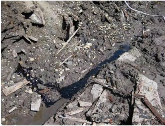
Photo 17B: BRPH-like free product draining from north sidewall adjacent to south side of East 19 th Street UST looking northeast.
