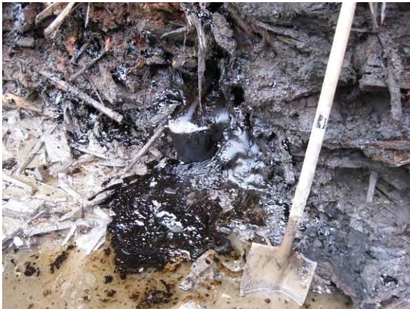
Photo 29C: BRPH free product – east sidewall below west entrance of Tacoma Fixtures bus building with shovel for scale.
