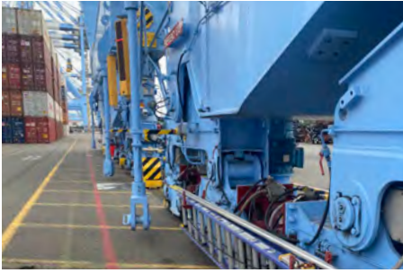
Crane tie-downs and stowage pins can be used to safely secure a crane in the event of strong winds.
