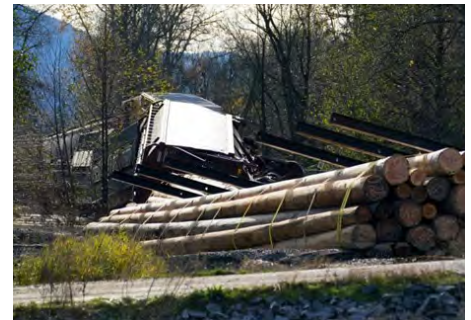
The November 2021 flood event was especially devastating for British Columbia, but it also affected goods movement in Washington. Damage to rail tracks caused the derailment of several railroad cars in Sumas, Washington.
