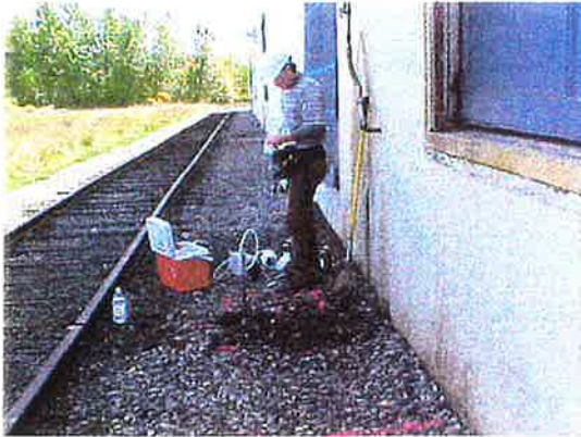
Water sampling at Boring B15.
