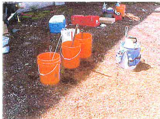
View of sequential decontamination wash sequence at the B1 boring location.
