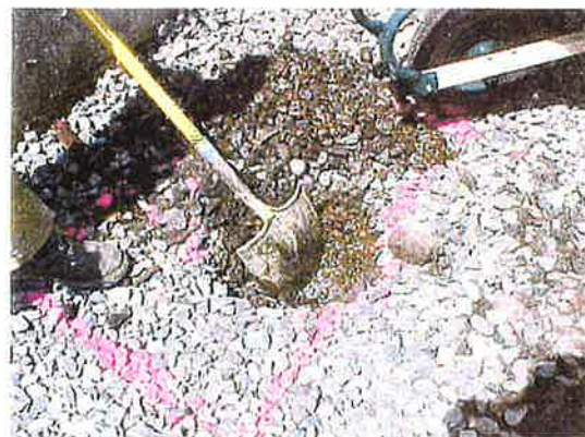
B15 location. After seeing the push probe coated with oil, a shovel was used to dig through the crushed rock aggregate. A significant thickness of free product was present, which flowed out of the aggregate toward the center of the hole.
