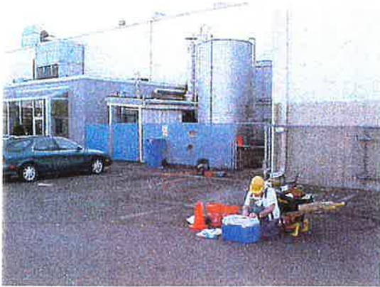
West side of REXAM plant. Groundwater sampling in Boring B4 in progress; B3 boring location near blue fence in distance.
