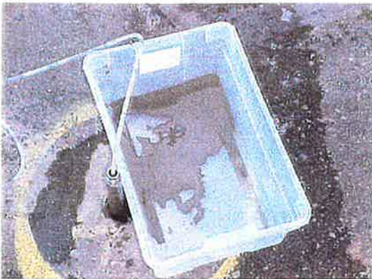
A peristaltic pump and clean polyethylene hose were used to pull water out of the temporary well point.
