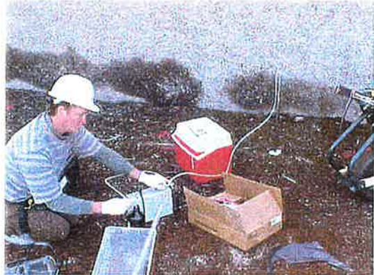
Groundwater sampling of Boring B1 in progress. Water samples were placed in cooled storage immediately after sealing.
