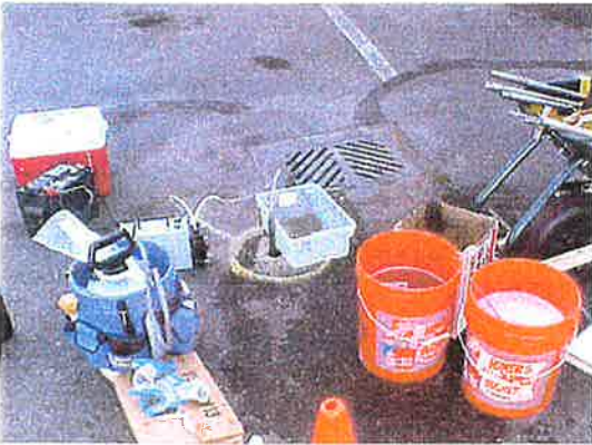
B4 sampling location was near catch basin in paved area of site. Decontamination procedure was performed with sequential wash sequence concluding with rinse of distilled water (in sprayer).
