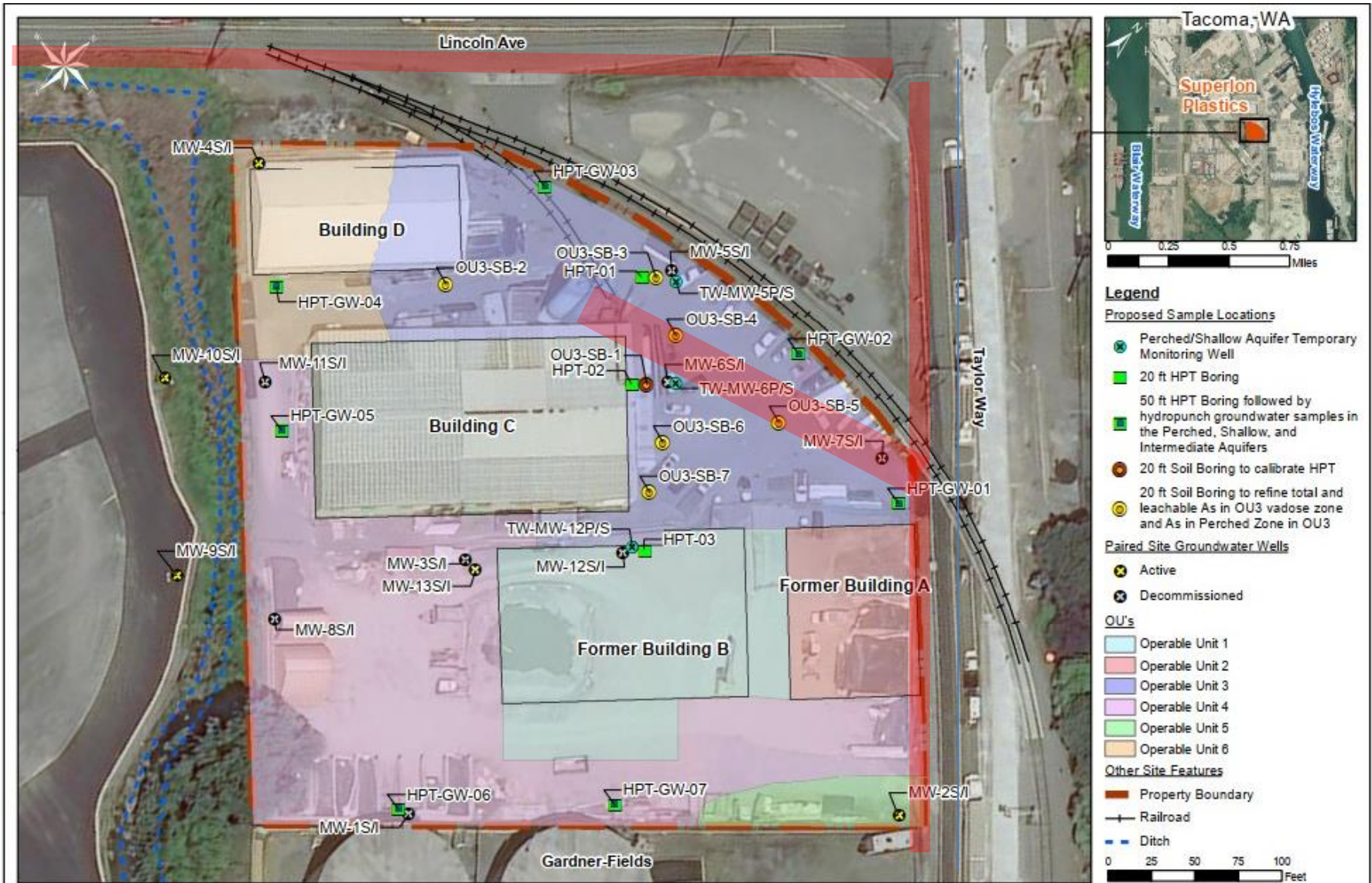
Proposed Sample Locations Remedial Investigation Phase V Work Plan Superlon Plastics Property, Tacoma, Washington
