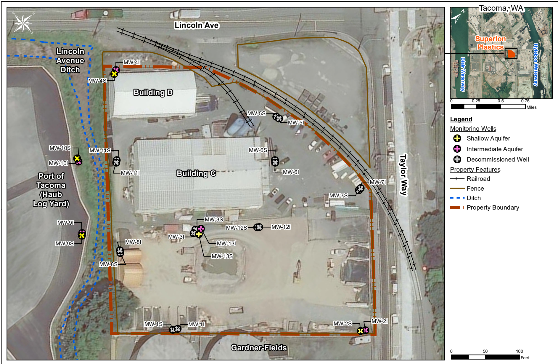
Monitoring Well Locations Remedial Investigation Phase V Work Plan Superlon Plastics Site, Tacoma, Washington
