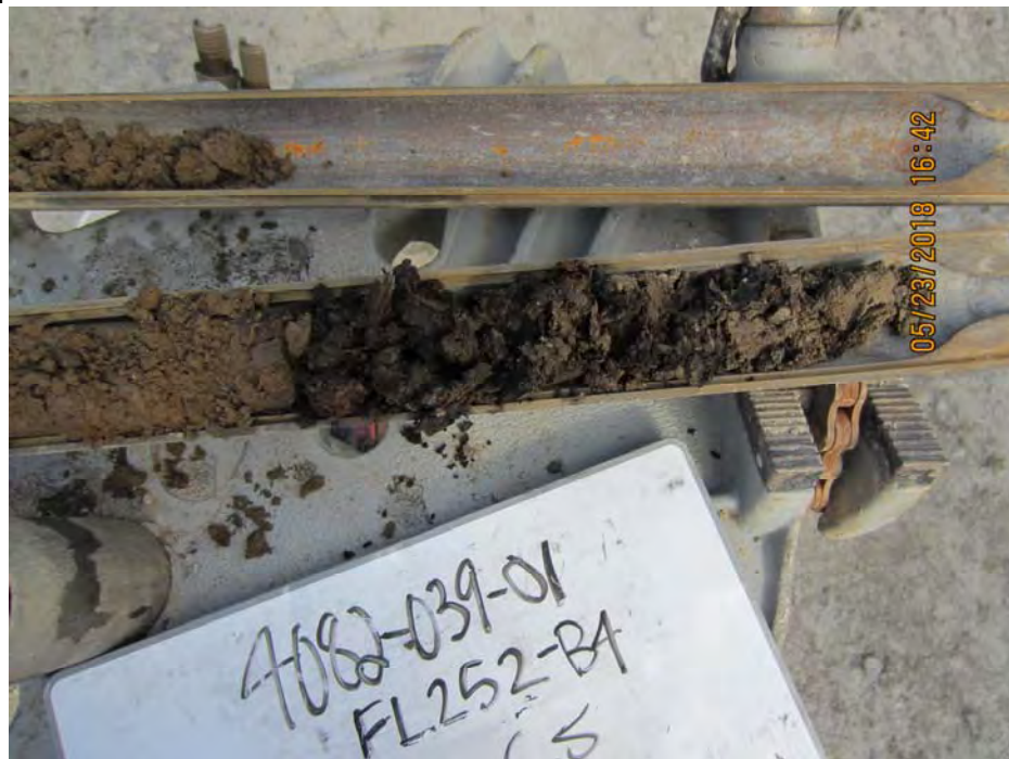
Photograph 8 – FL-252 – Exploration FL252-B4 soil core from 5 to 6.5 feet below ground surface. The dark layer contained wood chunks. Lube oil-range petroleum hydrocarbons were detected in this sample at a concentration greater than the MTCA Method A cleanup level.
