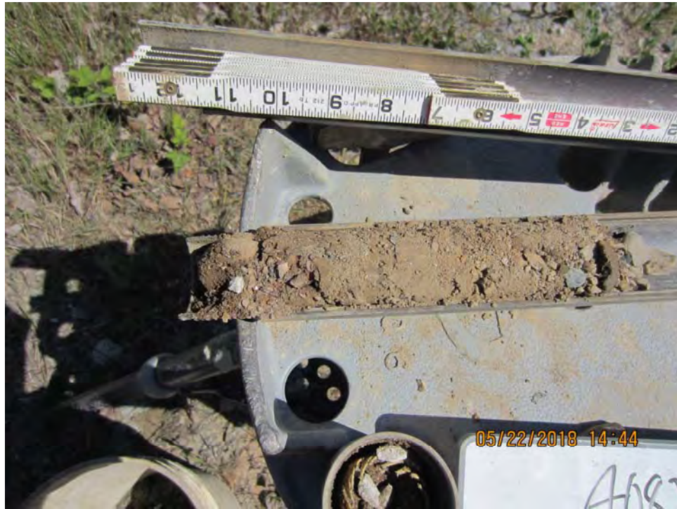
Photograph 7 – FL-252 – Exploration location FL252-B1 soil core from surface to 1.5 feet below ground surface. Arsenic and cPAHs were detected in this sample at concentrations greater than corresponding MTCA cleanup levels.
