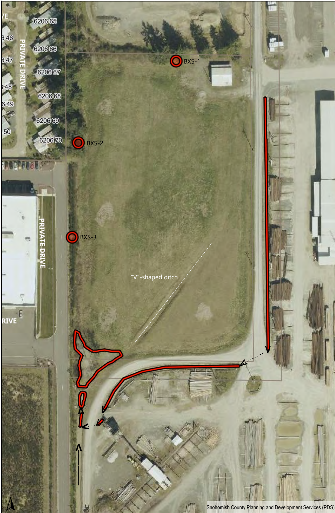
Figure 2. Baxter South woodwaste landfill, stormwater routing to infiltration basin.
