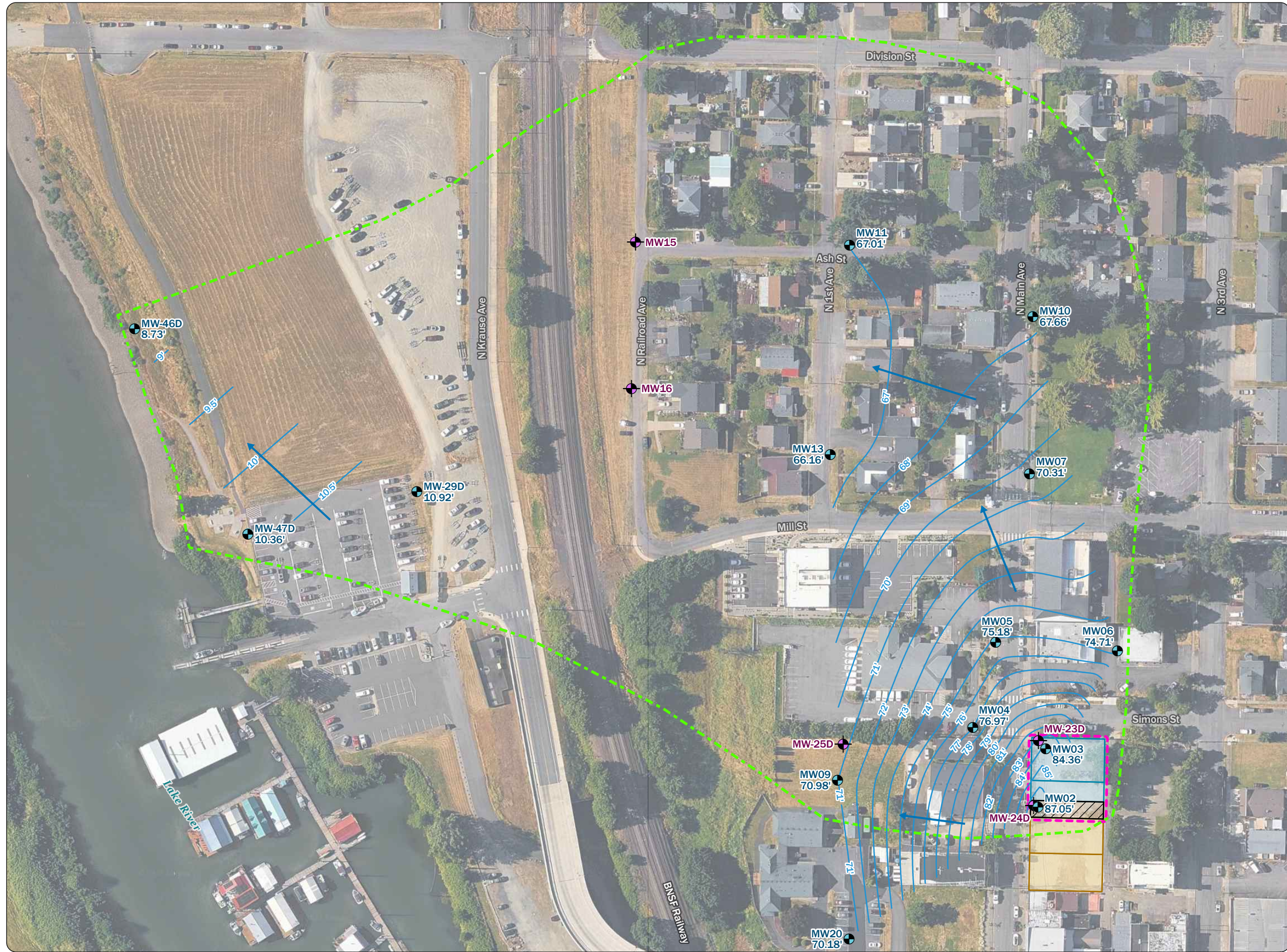
Figure 2 Estimated Upper-Water Bearing Zone Groundwater Potentiometric Surface Map December 2025 Former Park Laundry Ridgefield, WA
