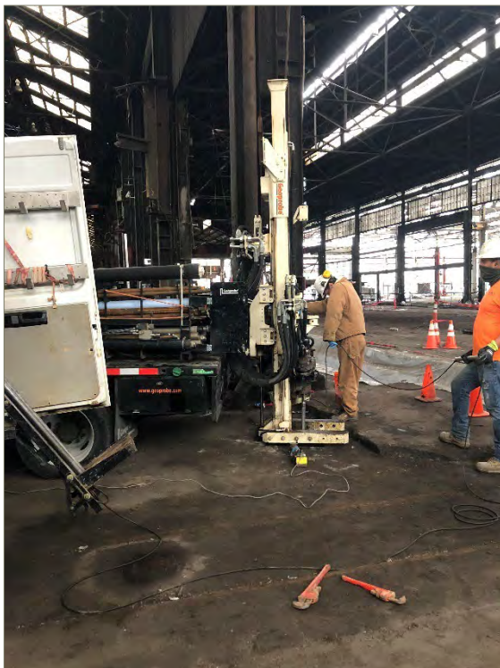
Exhibit C-2: Photo of the Direct-Push Drill Rig Used for the LIF Investigation
