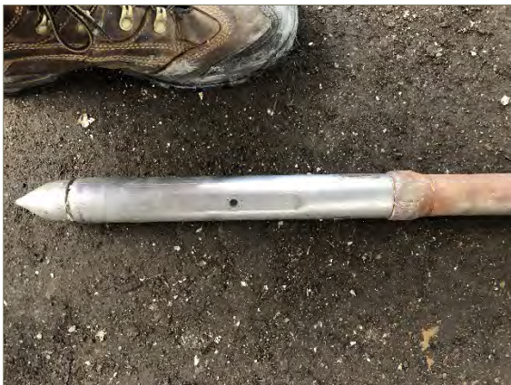
Exhibit C-1: Photo of a Direct-Push Probe with Transparent Window Used for the LIF Investigation
