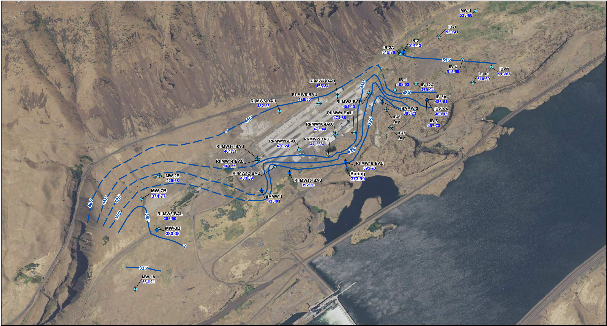
Figure 12 Potentiometric Surface for Uppermost Basalt Aquifer Groundwater Wells Remedial Investigation / Feasibility Study Goldendale Energy Storage Project Goldendale, Washington
