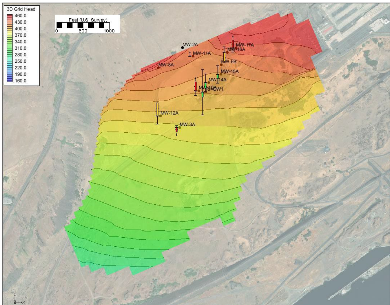
Figure 10. Calibrated water levels in the alluvium.
