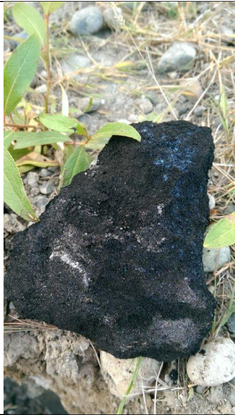
Photograph: 7 Carbon material from sidewall with blue hue from copper
