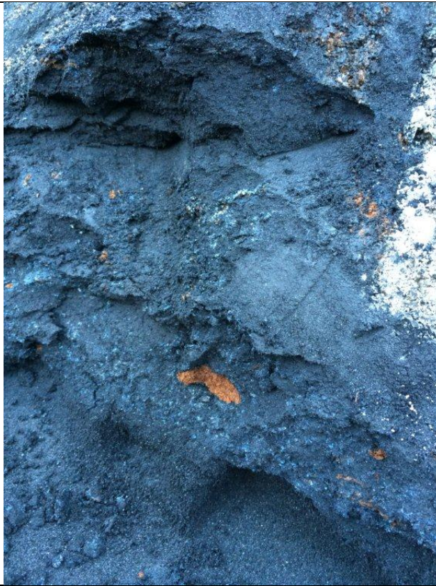
Photograph: 3 Soil horizon includes sawdust, black carbon and blue color from copper
