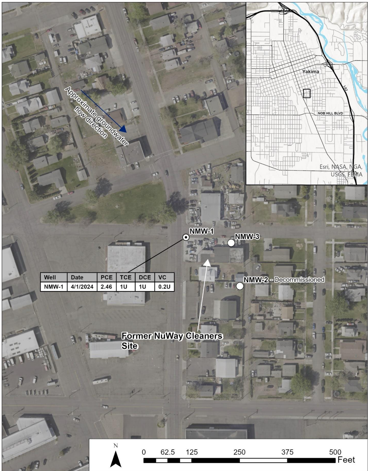
Figure 4. Nu-Way Cleaners Well Locations and cVOC Results ( \mu\text{g/L} ), 2024.
