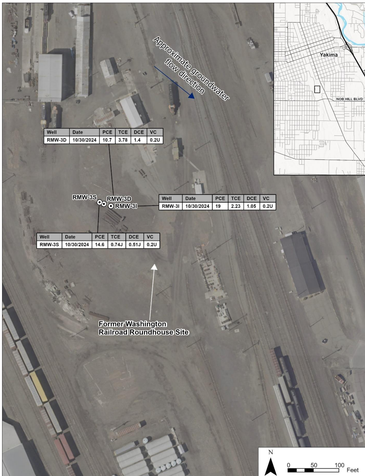
Figure 6. Washington Central Railroad Roundhouse Well Locations and cVOC Results ( \mu\text{g/L} ), 2024.
