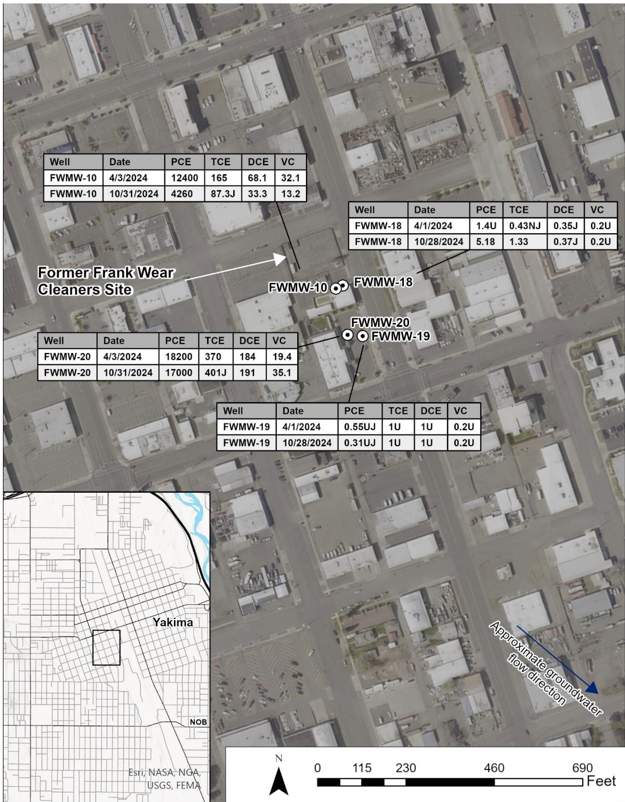
Figure 9. Frank Wear Cleaners Well Locations and cVOC Results ( \mu\text{g/L} ), 2024, 2 of 2.
