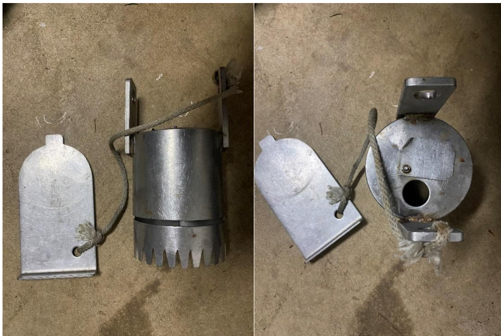
Figure 2. Four-inch stainless steel hand corer
