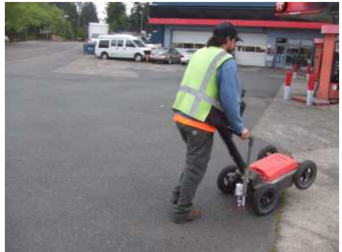
Photo 8. View of the GPR survey.
