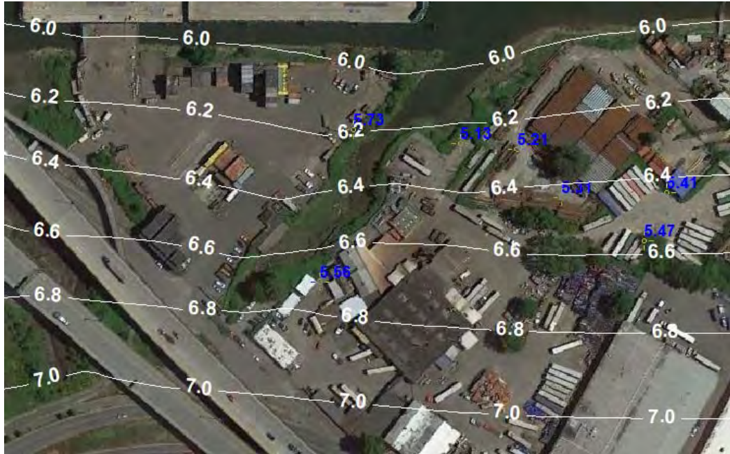
Figure 16. Model water level contours for the lower sand unit (model Layer 4)
