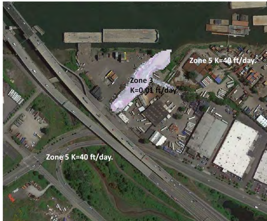
Figure 8. Horizontal hydraulic conductivity zones in model Layer3.
