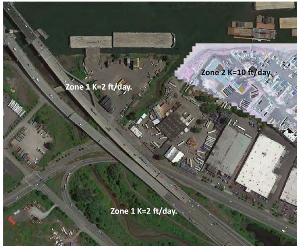
Figure 6. Horizontal hydraulic conductivity zones in model Layer 1.
