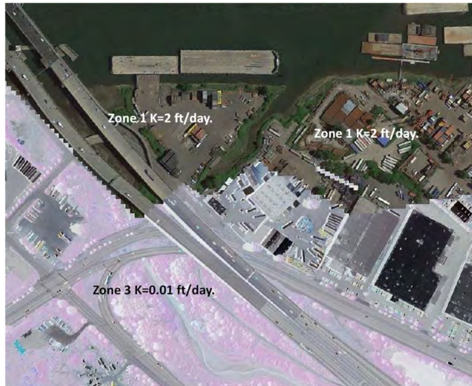
Figure 7. Horizontal hydraulic conductivity zones in model Layer2.
