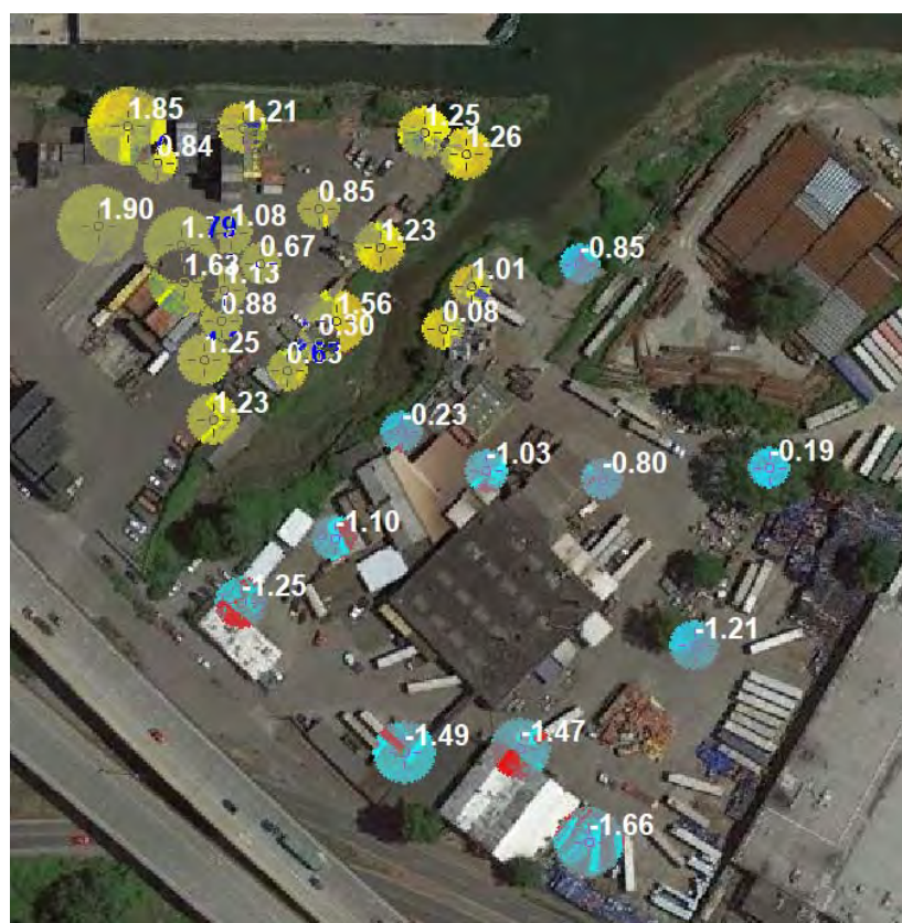
Figure 13. Water level residuals (ft) for the lower sand unit (model Layer 3)
