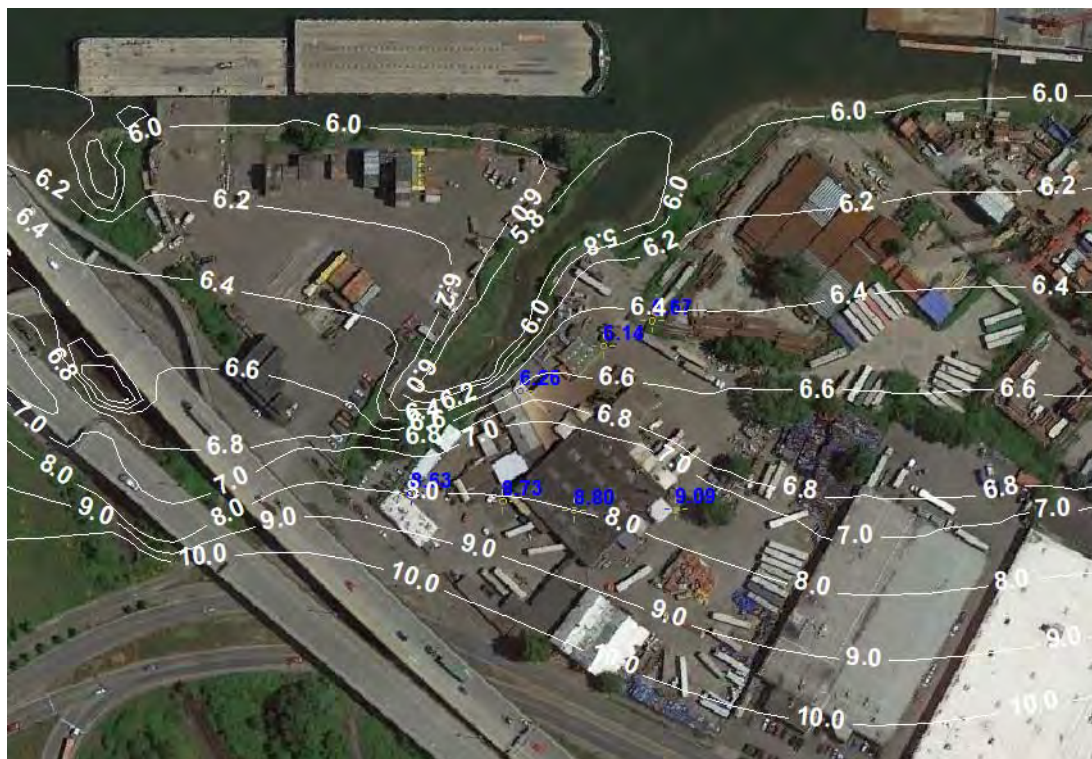
Figure 15. Model water level contours for the upper sand unit (model Layer 1)
