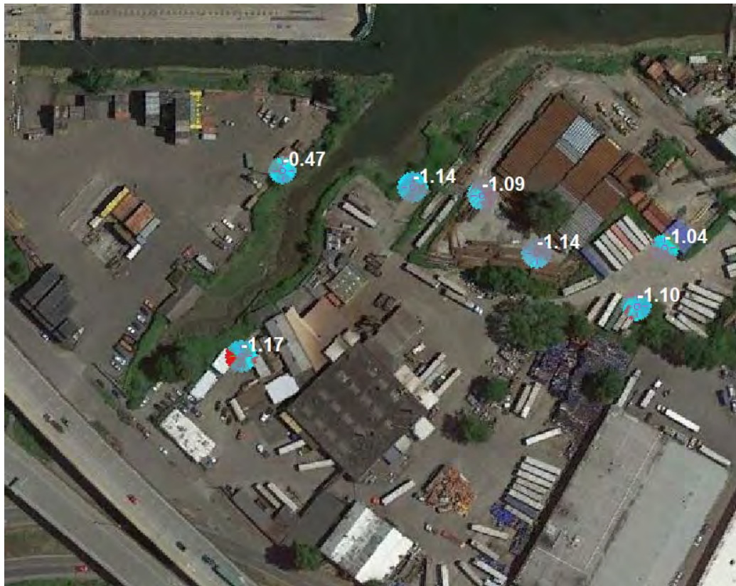
Figure 14. Water level residuals (ft) for the lower sand unit (model Layer 4)
