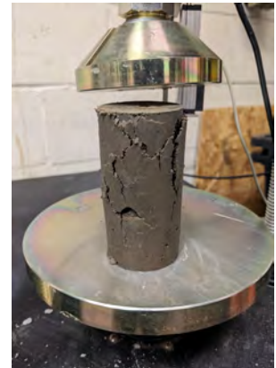
Sketch of Specimen After Failure
