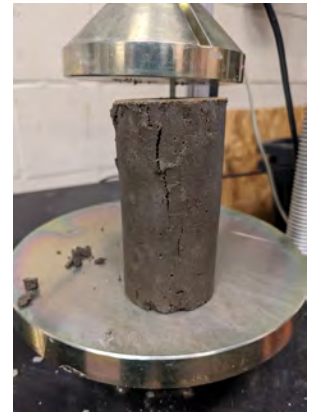
Sketch of Specimen After Failure
