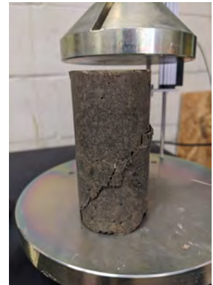
Sketch of Specimen After Failure
