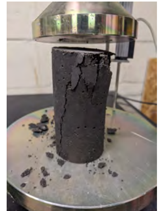
Sketch of Specimen After Failure
