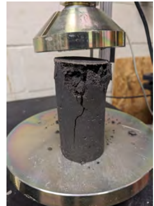
Sketch of Specimen After Failure
