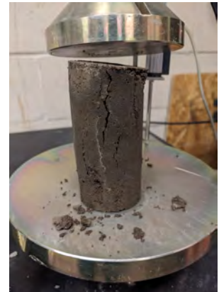
Sketch of Specimen After Failure
