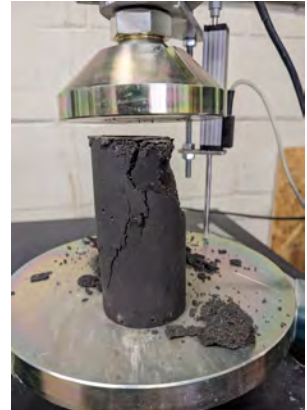
Sketch of Specimen After Failure
