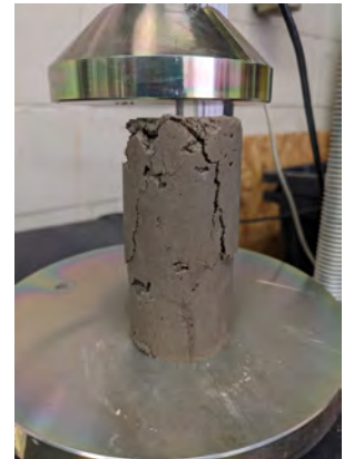
Sketch of Specimen After Failure
