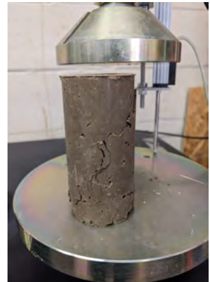
Sketch of Specimen After Failure
