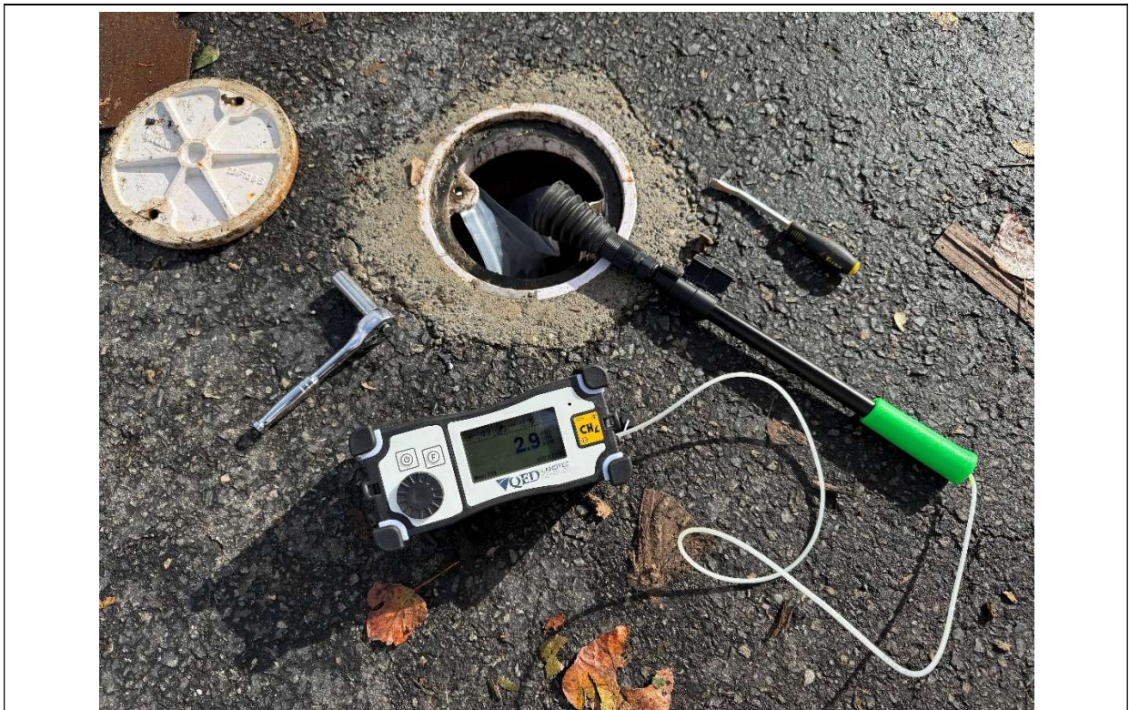
Landtec SEM5000 reading methane emissions at GP-32S monument. Methane concentrations at or below background measurements of 3.0 parts per million.
