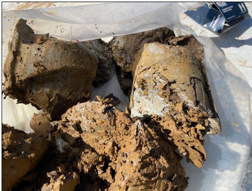
Photograph B-6. Tight/dense clay encountered at CBV-4483-07
