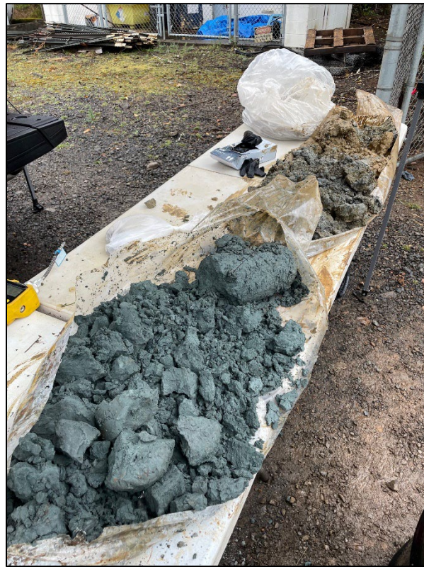
Photograph B-4. Tight/dense clay encountered at Wash Racks 1 and 2 location CBV-WR12-06
