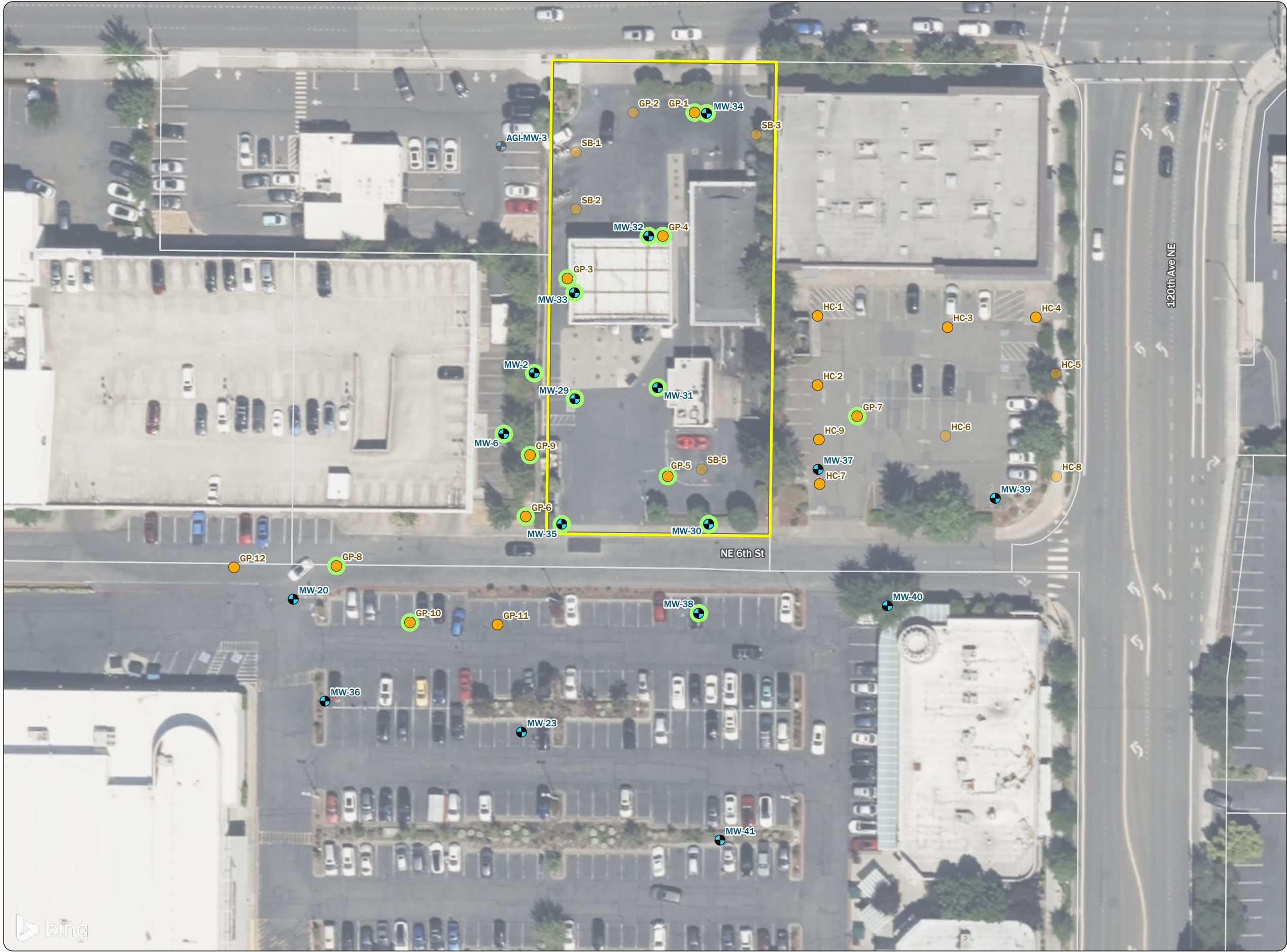
Figure 3-2 DRO+ORO Exceedances in Groundwater
