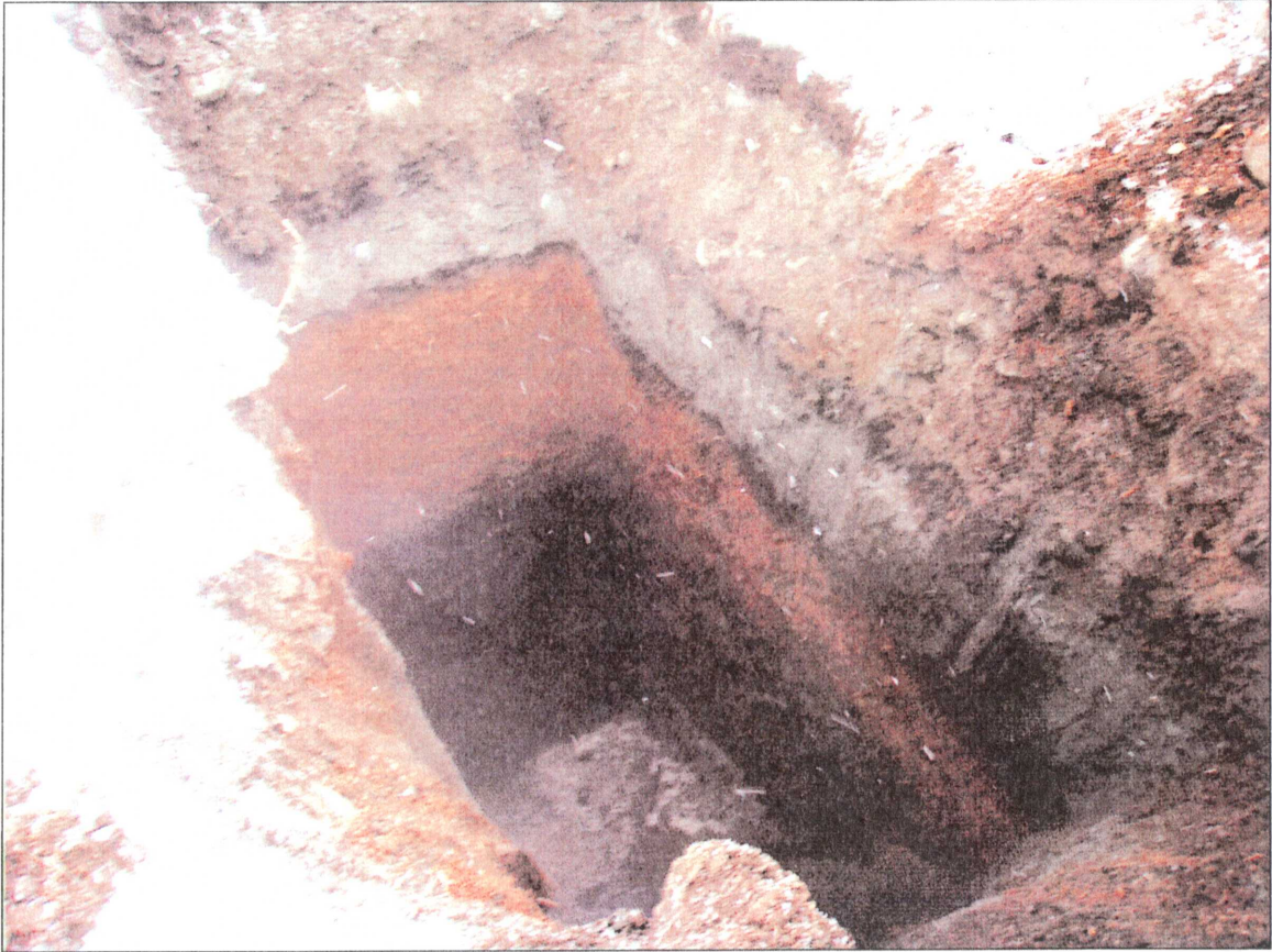
Figure 5. Imported soil overlying wood waste fill in Test Pit No. 1 located at the former site of the mill pond, near the intersection of Mill Road and Sunset Highway. Depth of test pit is 12 feet. Groundwater was encountered at a depth of 11 feet.
