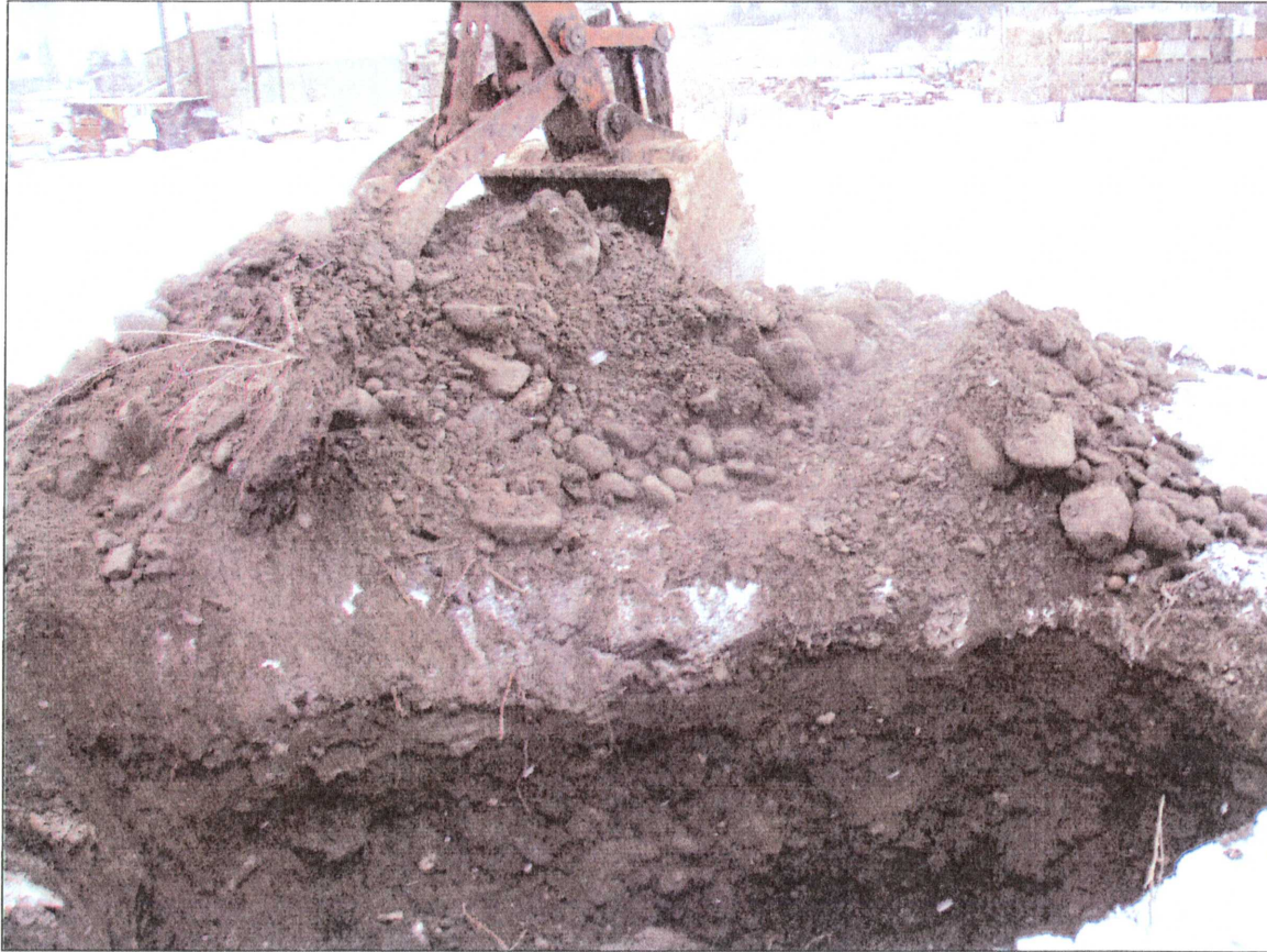
Figure 4. Alluvium consisting of poorly sorted sand, gravel and cobbles in Test Pit No. 3, located at the former site of the mill offices, approximately 50 feet south of Sunset Highway. Depth of test pit is 6 feet. Groundwater was encountered at a depth of 6 feet.
