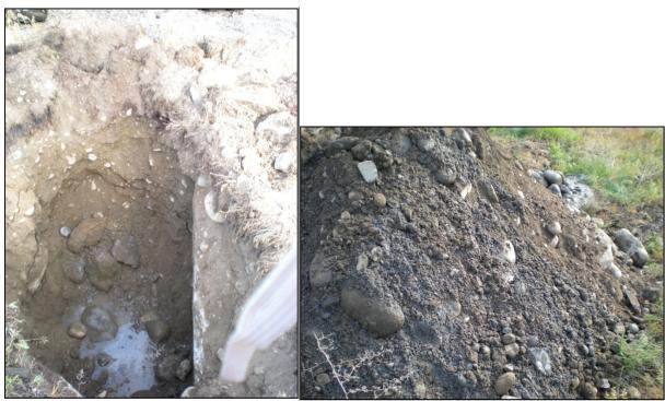
Photo 1 – Test Pit at Discovery Site (Depth = 6 ft); Photo 2 - Soil at Discovery Site
