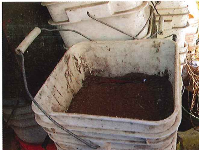
Fine material, reported to be metal byproduct from the lead melting operation.
