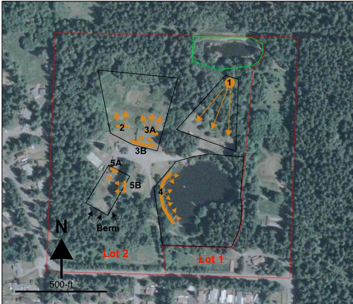
Figure 16. Map showing locations of proposed Active Shooting Range Management Areas (4 black polygons); shooting locations (1, 2, 3A, 3B, 4, 5A, 5B); shooting directions (orange arrows); Lower Pond Management Area (green polygon), and Lots 1 and 2 (red polygons). There are berms located at the south and southeast sides of Management Area 5. These berms prevent stray shot and bullets. The area outside of the black and green polygons in Lot 2 comprise the Non-Shooting Management Areas. The text describes BMPs and an institutional control for these management areas. Lot 1 will be managed separately and is excluded from these BMPs and institutional control.
