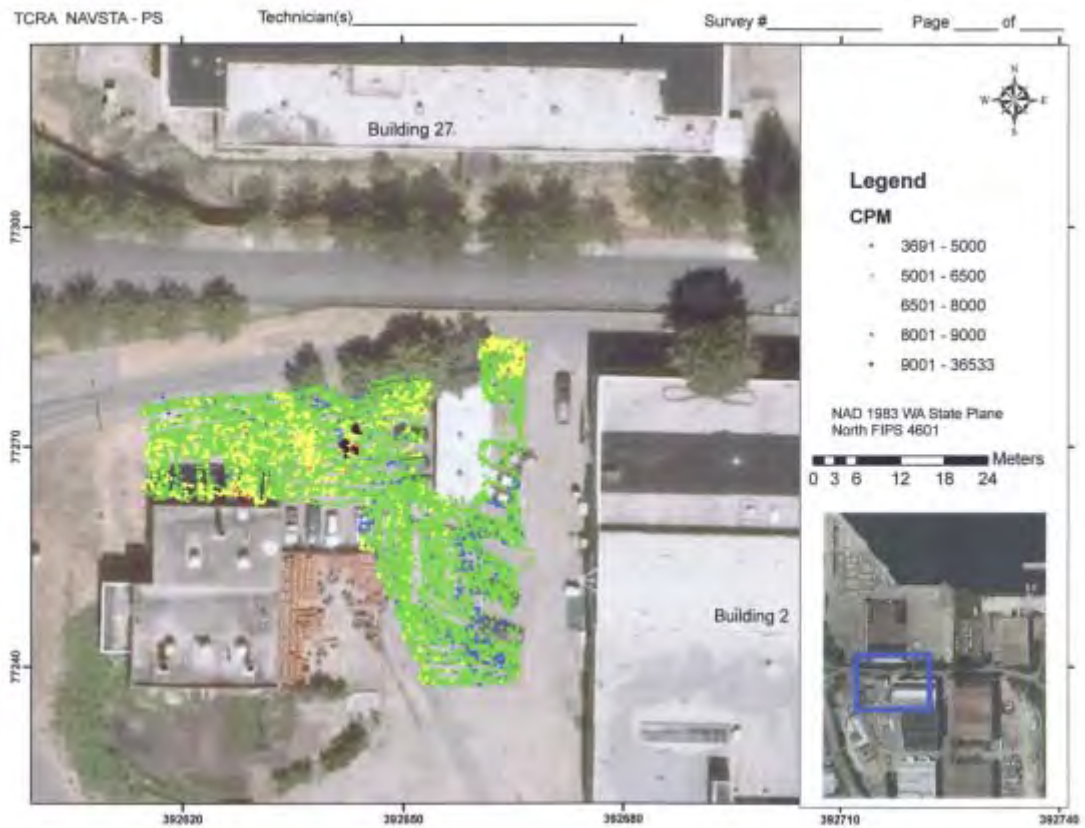
Figure 6 Gamma Walkover Survey - North of Building 12
