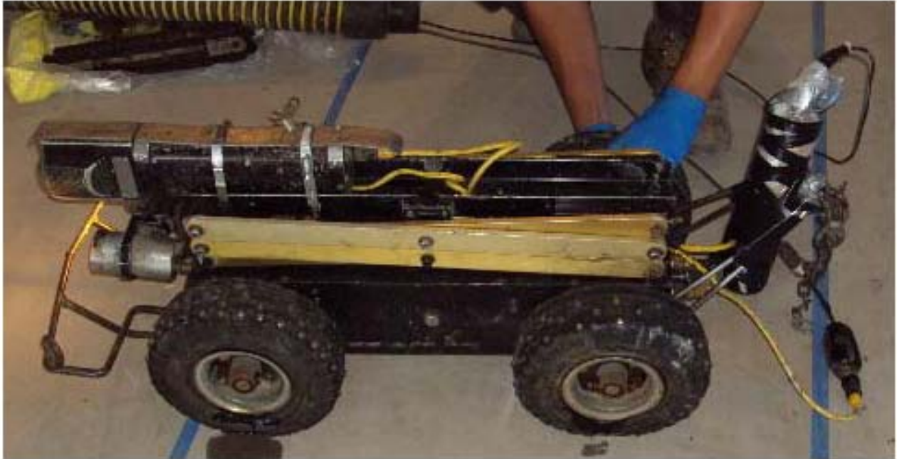
Figure 26 Tractor Coupled with Sodium Iodide 2 inch by 2 inch Detector
