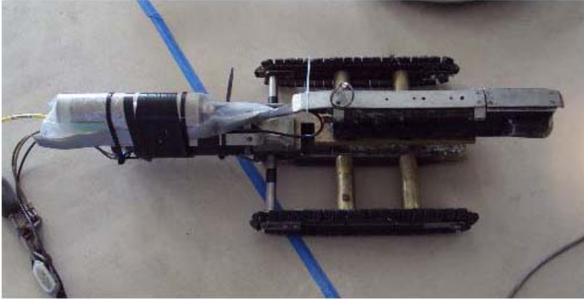
Figure 24 Pipe Crawler Coupled with Sodium Iodide 2 inch by 2 inch Detector
