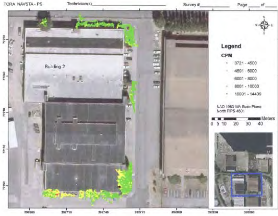
Figure 7 Gamma Walkover Survey - South and East of Building 2
