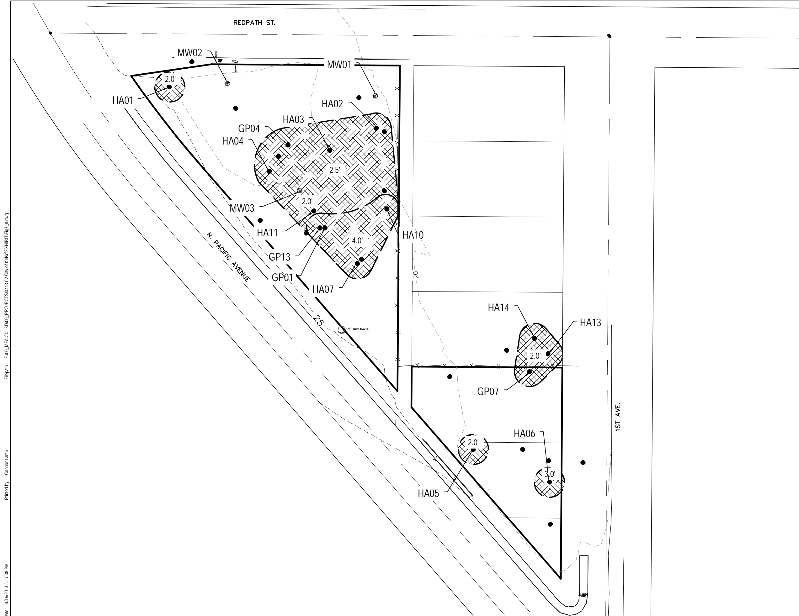
Figure 3 Alternative 1 Excavation of All Contaminated Soil
