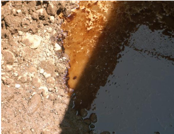
Photo #19: View of free product within test pit north 3 at approximately 5.5 feet below ground surface (bgs).
