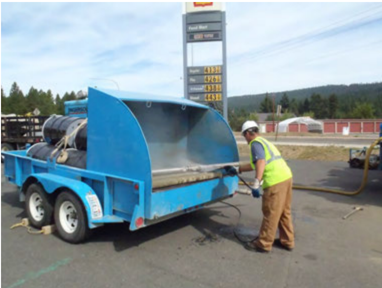
All drilling materials were decontaminated with pressurized water.
