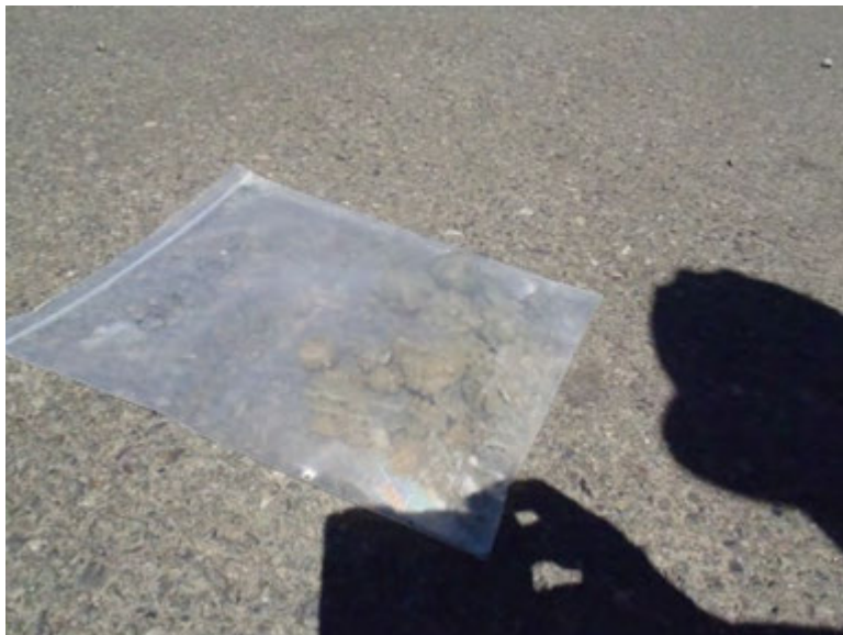
A portion of each sample was collected into plastic bags for field evaluation of volatile organic compounds using a Photo Ionization Detector (PID).
