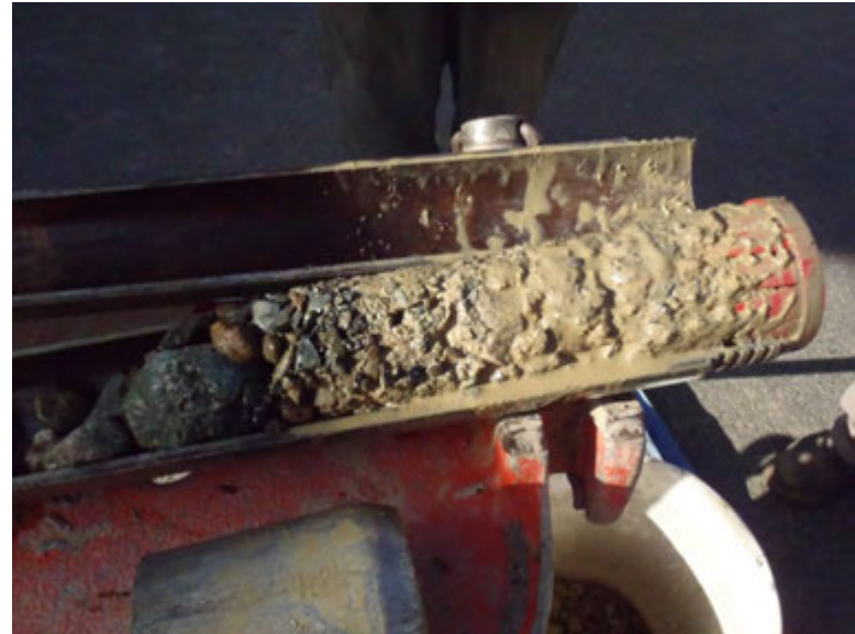
Samples were collected from each borehole with a split spoon core sampler.
