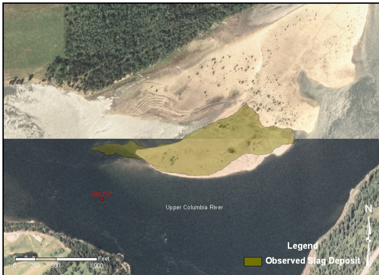
Figure 4: Survey area of observed slag deposit totaling approximately 20 acres in size.
