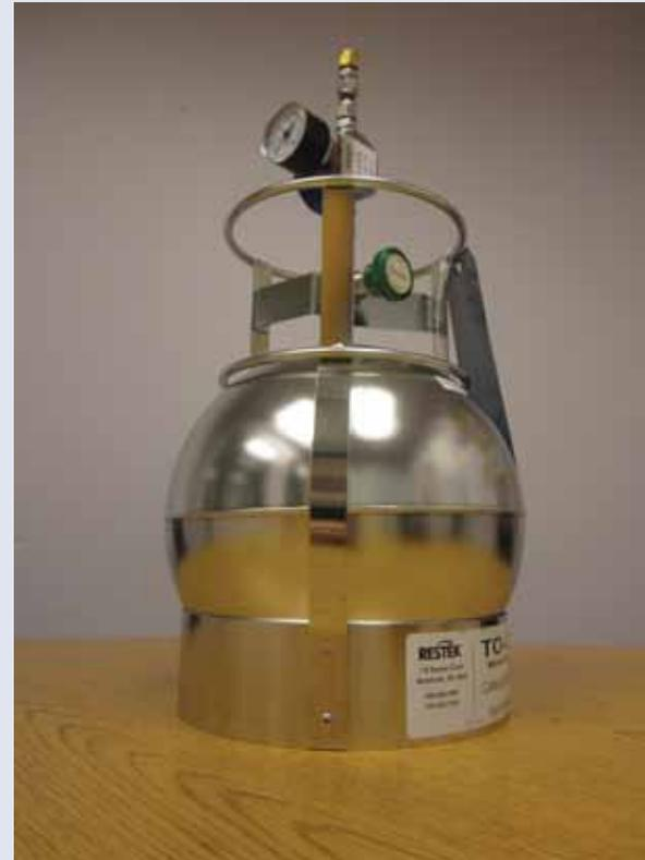
*Indoor air monitoring canister (approximately 18 inches tall) used for vapor intrusion testing*
