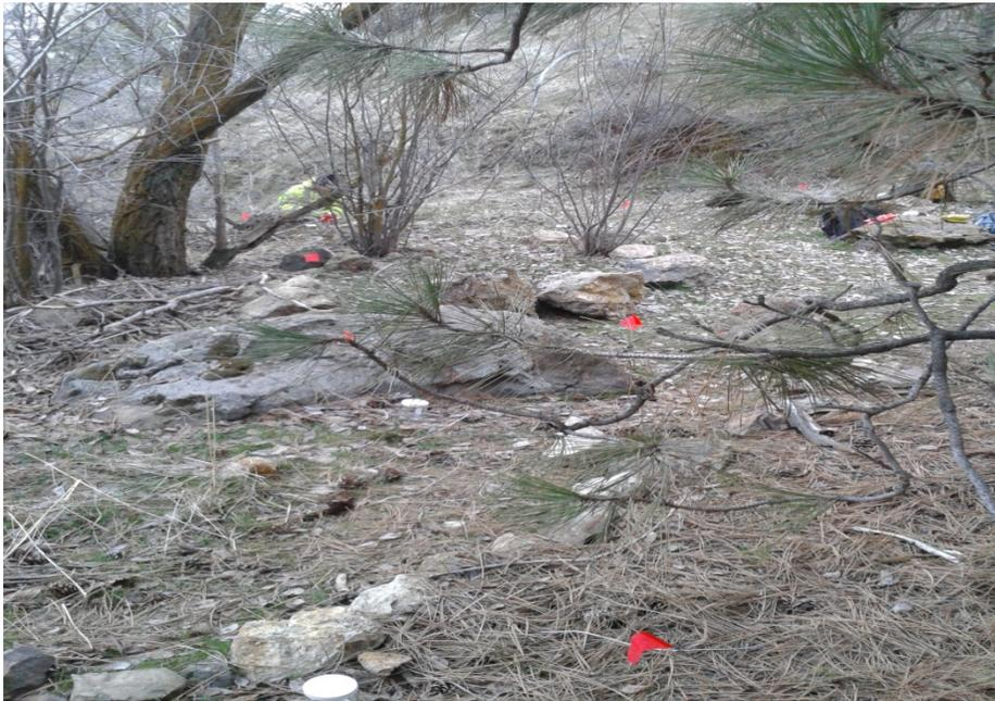
Photograph 3 – Flags marking a ten-point composite sample beyond the toe of waste rock pile at SR-01
