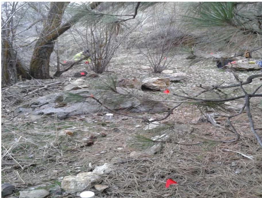
Photograph B-3 – Flags marking a ten point composite sample beyond the toe of the waste rock pile at SR-01.
