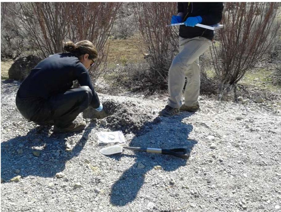
Photograph B-6 – Collecting a discrete sample from the waste rock pile at SR-02.
