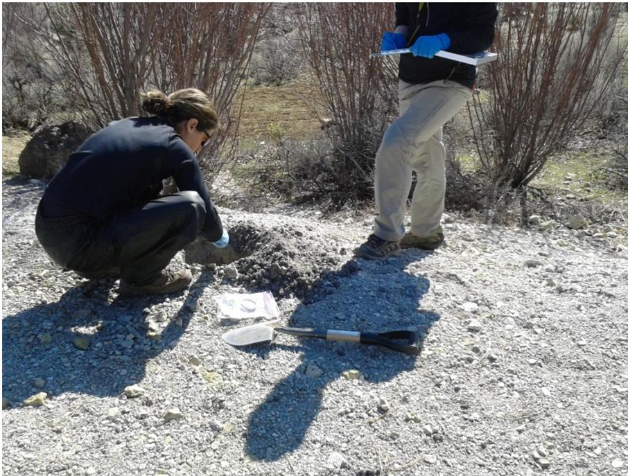
Photograph 6 – Collecting a discrete sample from the waste rock pile at SR-02.
