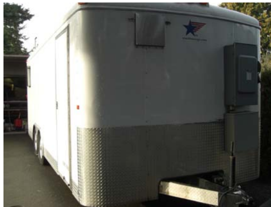
Front of 24' trailer featuring power supply boxes and sparge room exhaust fan
