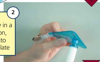
2 Keeping the diffusive body in a vertical position, to screw it onto the support plate
