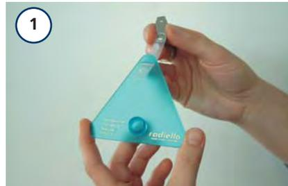
1 insert the clip strip in the slot, with the peg facing upwards
