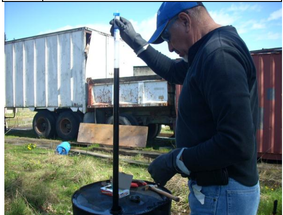
Photo #6: View of onsite drums being profiled for presence of solvents.
