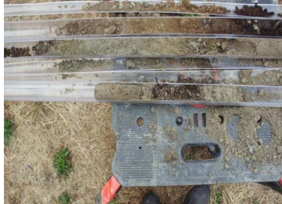
Photo #2: Soil profile from boring B-3 showing medium dense silty sand at surface (top right) which grades to stiff silt and very dense grey silty sand bottom right (refusal at 13 ft bgs)
