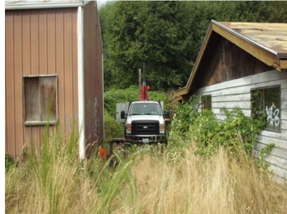
Photo #8: Direct push probe located at boring B-1 in the northwest portion of Parcel C where dumping of unknown materials occurred. View looking west.
