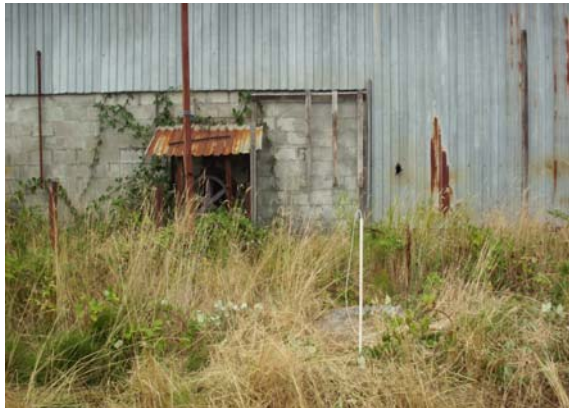
Photo #9: Temporary PVC screen placed in boring B-14 to attempt groundwater sampling in east central portion of Parcel A. Note: former auto body shop in background. View looking west.
