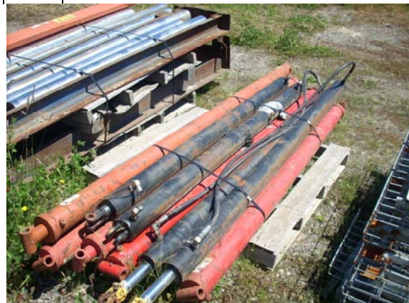
Photo #18: View of dismantled hydraulic hoist on south side of Parcel B.
