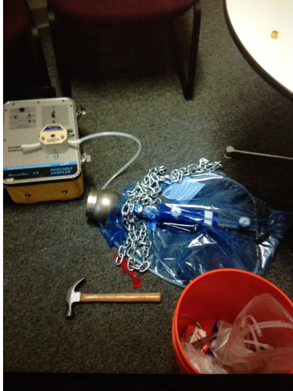
Photograph 19. Subslab sampling setup, November 2012.
