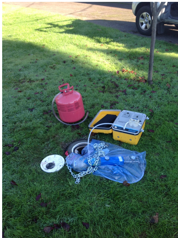
Photograph 14. Soil gas sampling setup, November 2012.
