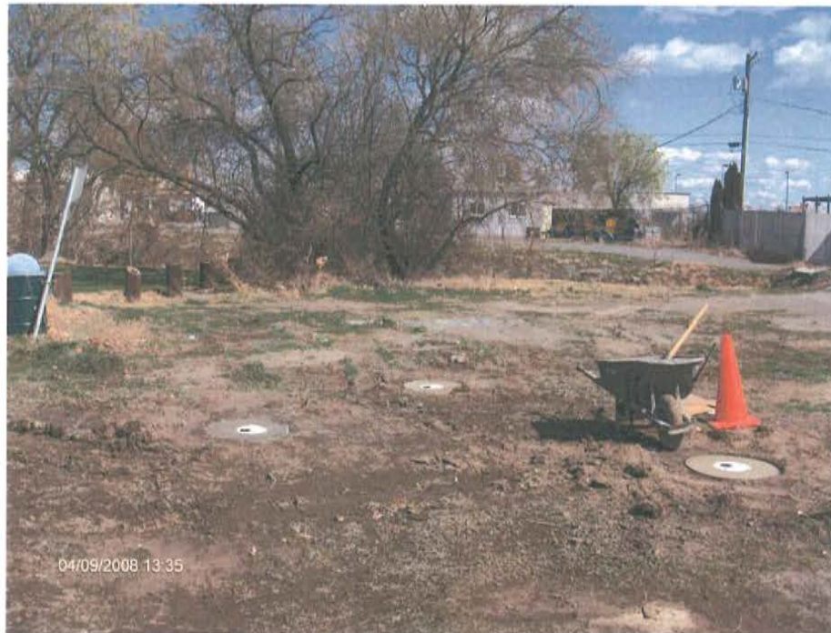
Photo 1: Photograph of monitoring wells MW-11s, MW-11I, and MW-11D located west of the New City Cleaner Site (photograph taken from the east).
