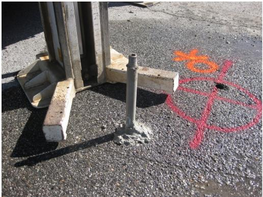
Photograph 12: View of combustible soil gas monitoring point SG4. Direct-push probe rods with a bentonite clay seal were used.
