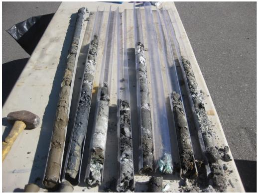
Photograph 19: View of the typical subsurface soil conditions at the Property in the vicinity of boring PZ3, located in the northwestern portion of the Property within the inferred footprint of the historical landfill.
