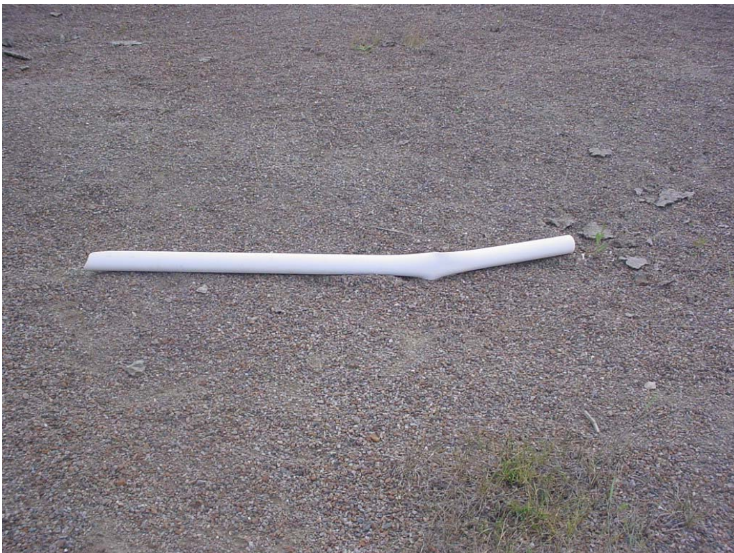
Photograph 4 - 2-inch-diameter, broken, white plastic pipe.
