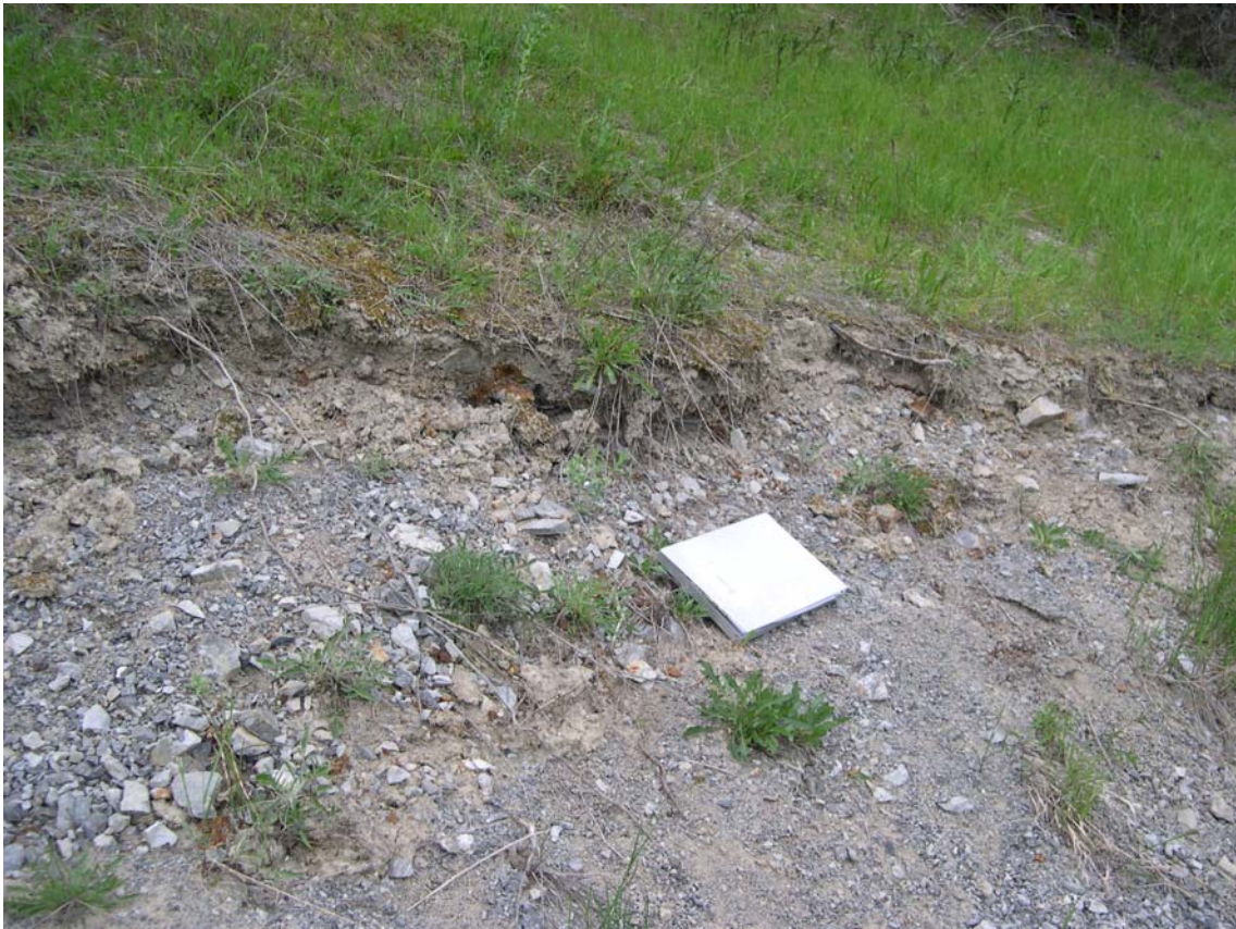
Photograph 2 - View of WR-1 waste rock mixed with river sediments in location of recent bank scour along Pend Oreille River.
