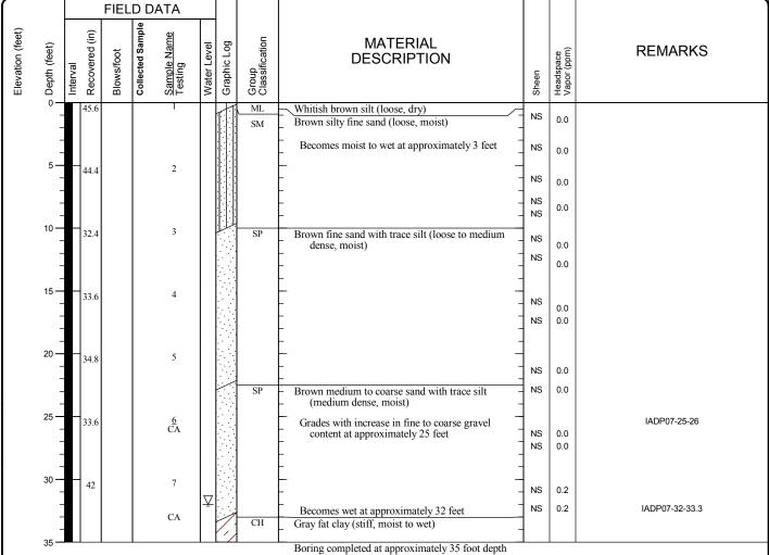
Boring completed at approximately 35 foot depth and backfilled with bentonite
