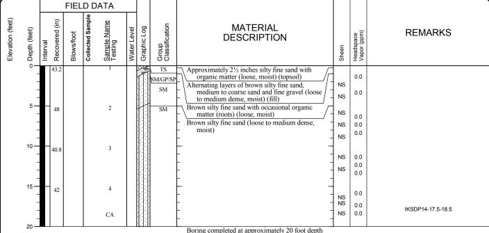
Boring completed at approximately 20 foot depth and backfilled with bentonite
