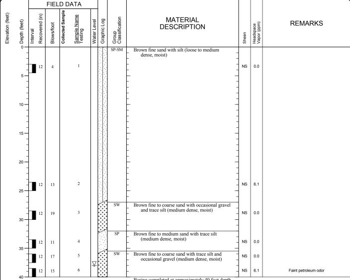
Boring completed at approximately 40 foot depth and backfilled with bentonite
