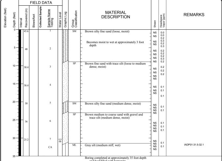
Boring completed at approximately 35 foot depth and backfilled with bentonite
