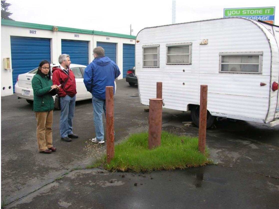
Monitoring well MW-16. Two wells clustered within the protective casing. Located approximately 400 feet SW of the source site.
