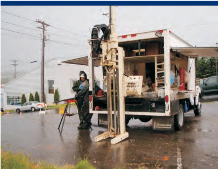
Photo 3 Drilling and sampling at JA05 at the former pest control business.
