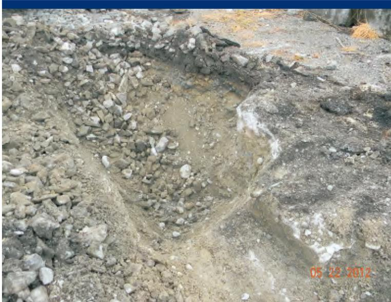
Photo 5 Test Pit 2 with building footings and 1-inch rebar.
