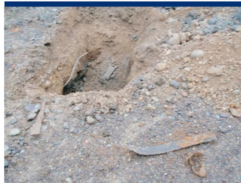
Photo 8 Test Pit 3 with rebar and metal scrap.
