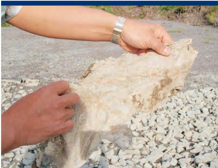
Photo 19 Photo of a piece of plastic liner that is present on the northeast corner of S. Jefferson Ave at former 2102 S. Jefferson Avenue. The plastic is below fill, then asphalt, and above concrete rubble.
