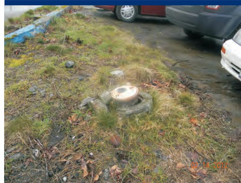
Photo 2 Monitoring well MW6 on east side of property.
