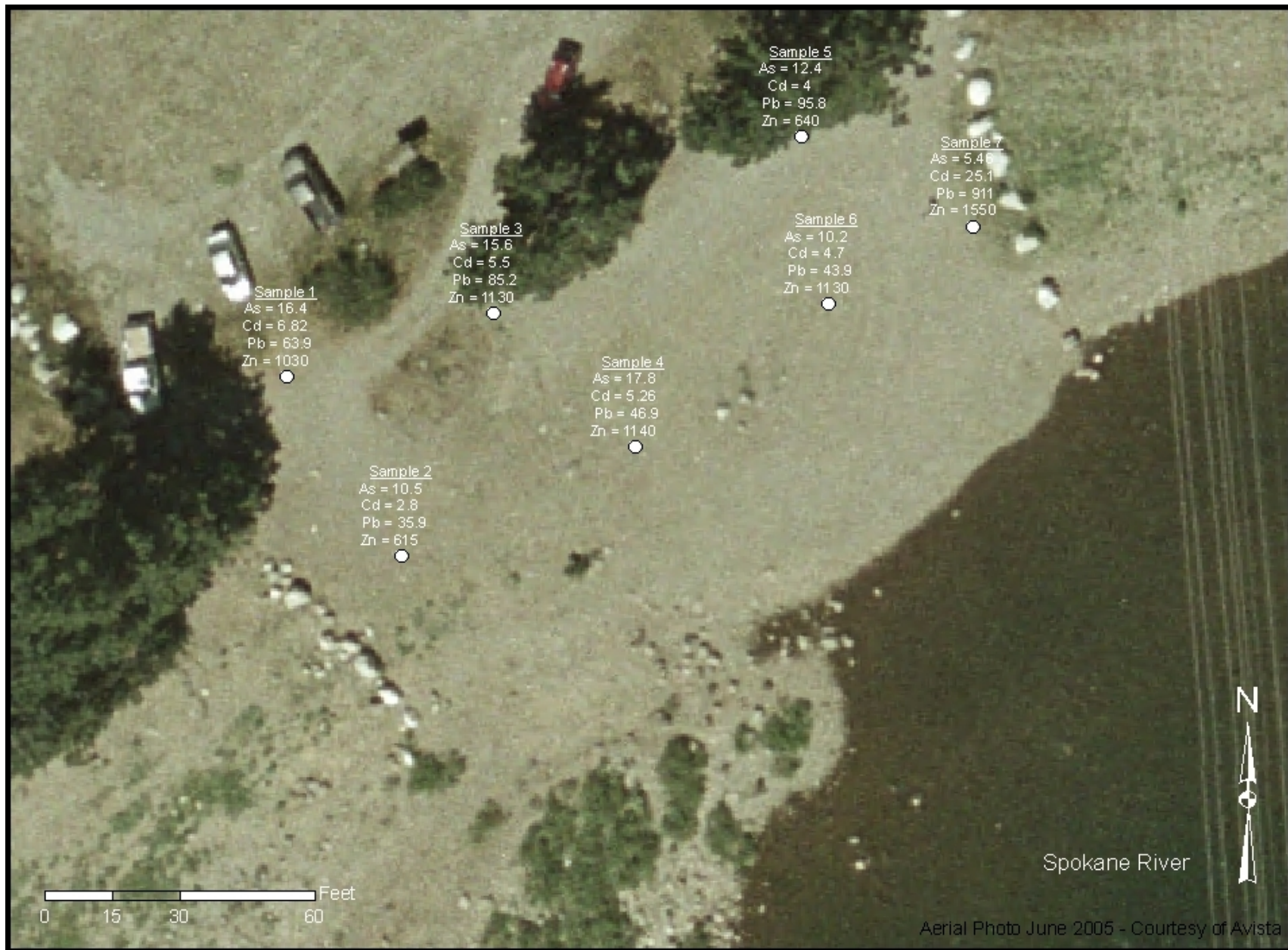
Figure 3. Laboratory Results of Samples collected at 1-foot nominal depth (all concentrations mg/kg)
