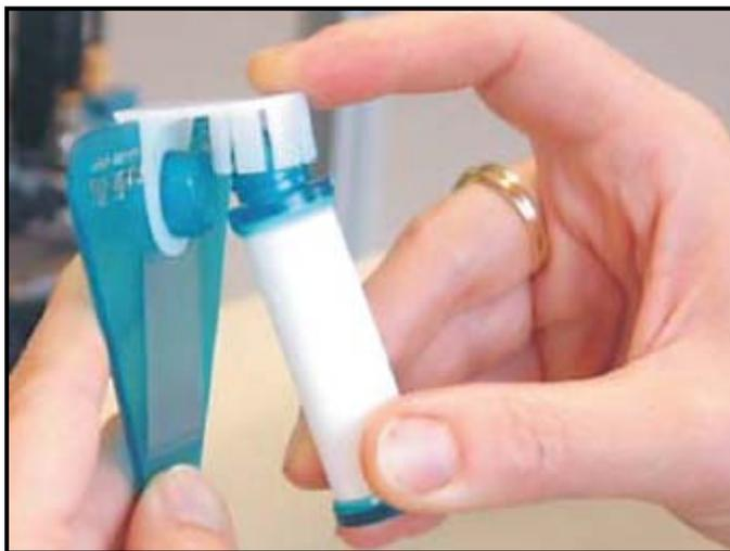
**Figure 6: Passive Diffusive Radiello Sampler**
