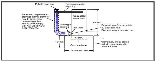
Figure 4.26 – Sediment Pond Riser Detail
