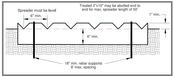
Figure 4.12 - Detail of Level Spreader
