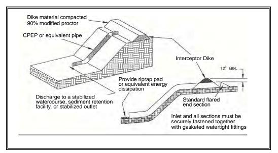
Figure 4.10 - Pipe Slope Drain
