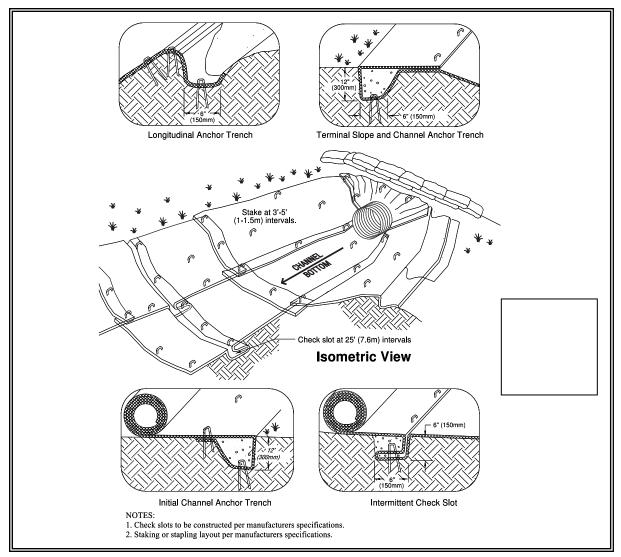
Figure 4.4 – Channel Installation
