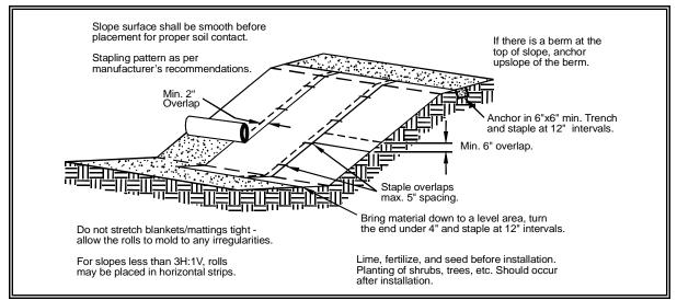
Figure 4.5 – Slope Installation
