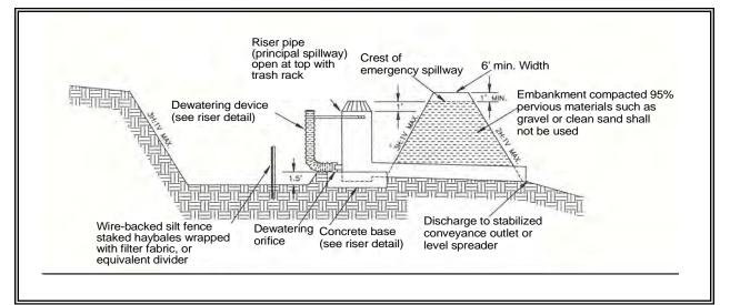
Figure 4.25 – Sediment Pond Cross Section
