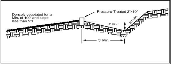
Figure 4.11 – Cross Section of Level Spreader
