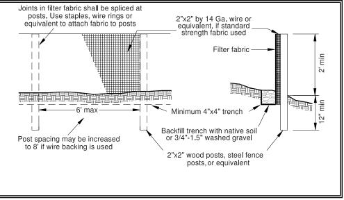
Figure 4.19 – Silt Fence
