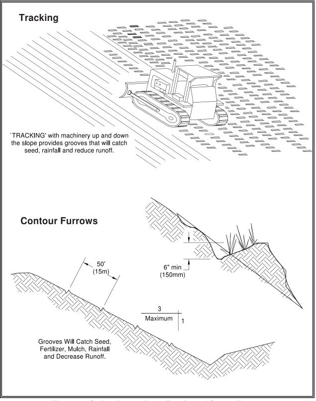
Figure 4.6 – Surface Roughening by Tracking and Contour Furrows
