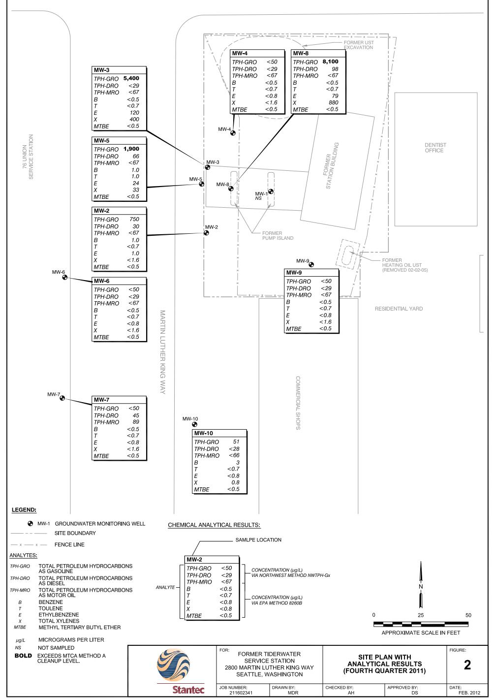
FILEPATH:M:\Tidewater\SEATTLE\2011\4th\TIDEWATER-SEATTLE\_F2-GWA.dwg | Layout Tab: 11x17L | Drafter: miramirez | Apr 19, 2012 at 13:41
